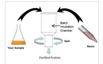
There is no resin carry-over to subsequent downstream analyses, no messy transfer of samples/resin slurries and negligible hold-up volume. As the device is contained, it is ideal for handling biohazardous samples and samples from infectious sources.
